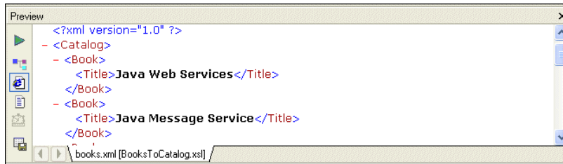
Figure 51. Result of Applying XSLT to books.xml
